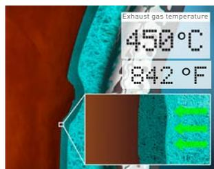
ISOLITE XP during heating: fibre insulation reaches activation temperature, the expansion process begins
