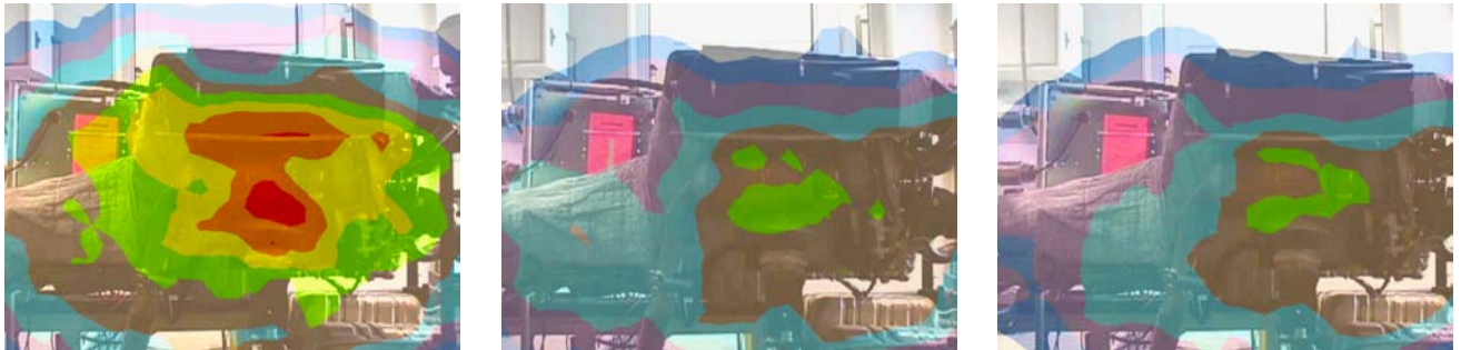
Near-engine noise absorption with positive thermal effects (l-r: without insulation, with 5 mm, with 10 mm).
